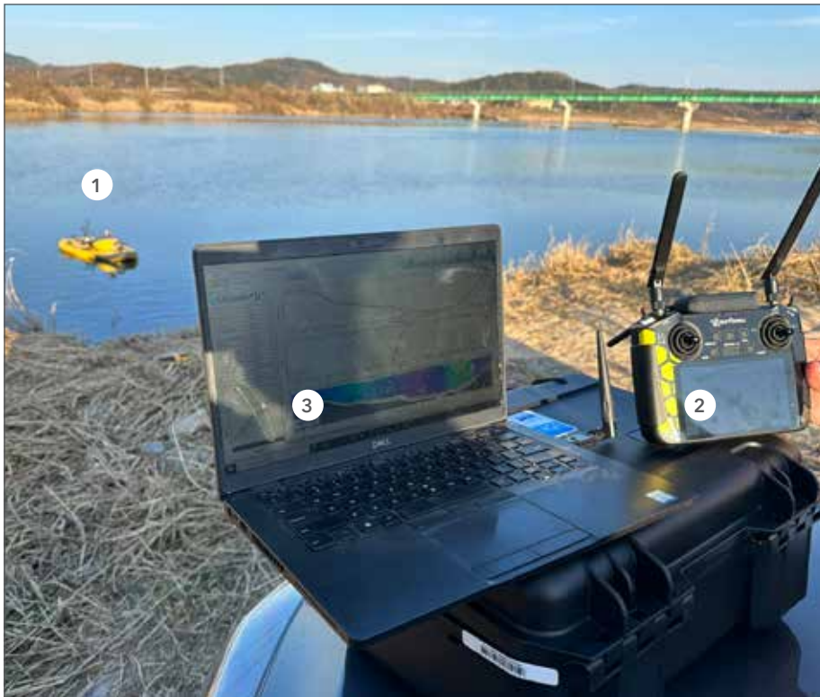
Figure 1: Surfbee Flow Seeker Conducting Discharge Measurement using ADCP Mode
