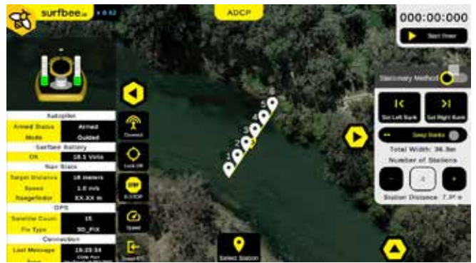
Figure 6: Setting the Number of Stations for a Stationary Measurement
