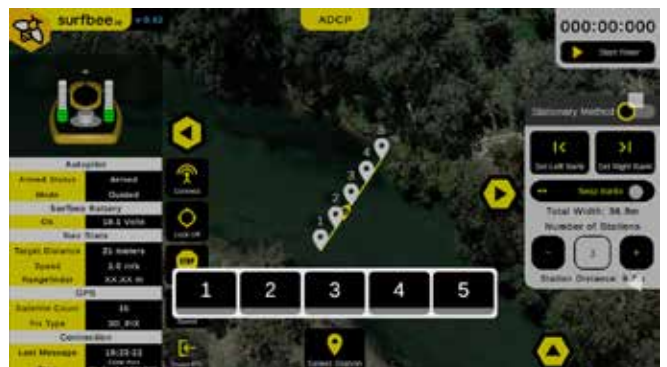
Figure 7: Directing Boat to a Station to Hold Position
